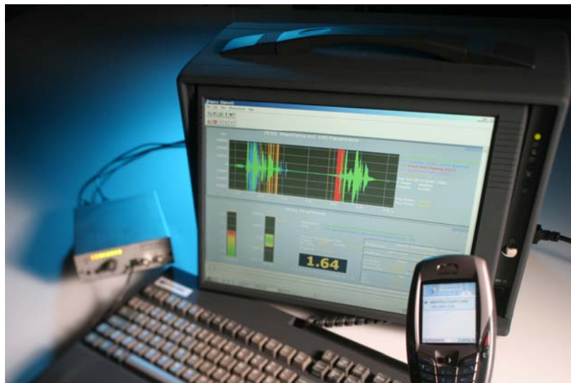
Figure 7-1 The OPTICOM OPERA Voice/Audio/Video Quality Analyser, offering PESQ, PSQM, PEAQ and soon also 3SQM and PEVQ analysis.
