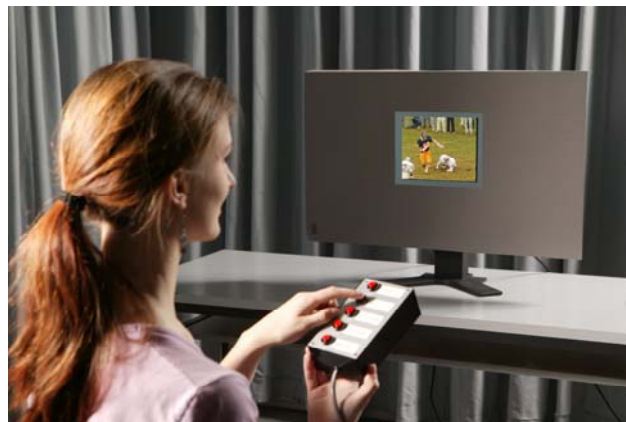
Figure 4-1 Viewing test room at the University of Erlangen where OPTICOM conducted subjective tests. The test subject watches a scene on an adjusted TFT screen from a well defined distance. By pressing one of the keys, the test subject will be able to score the scene on the 5 point opinion scale.
